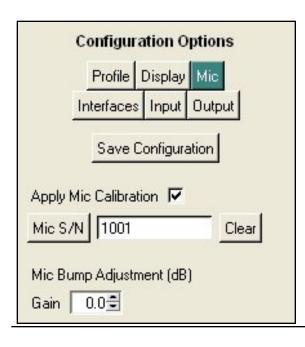
Enable and load microphone calibration file.
