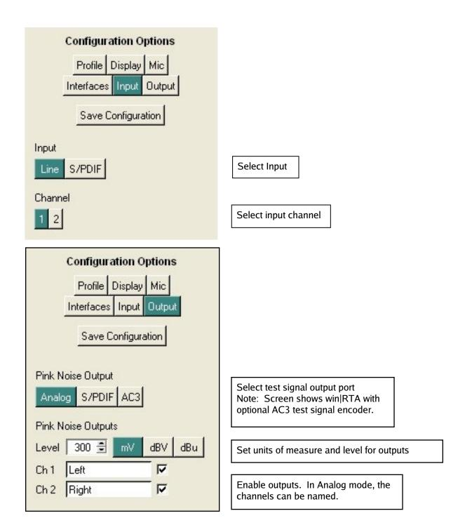
NOTE: The functionality shown on these screens will vary depending on the audio interface. Output voltage will only be correct with an approved interface.
