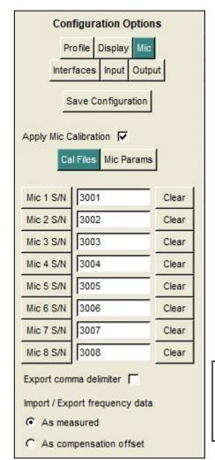
Enable and load microphone calibration files.
