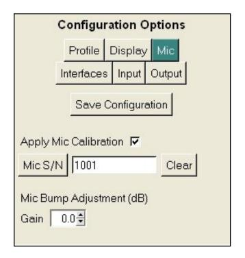
Enable and load microphone calibration file.
