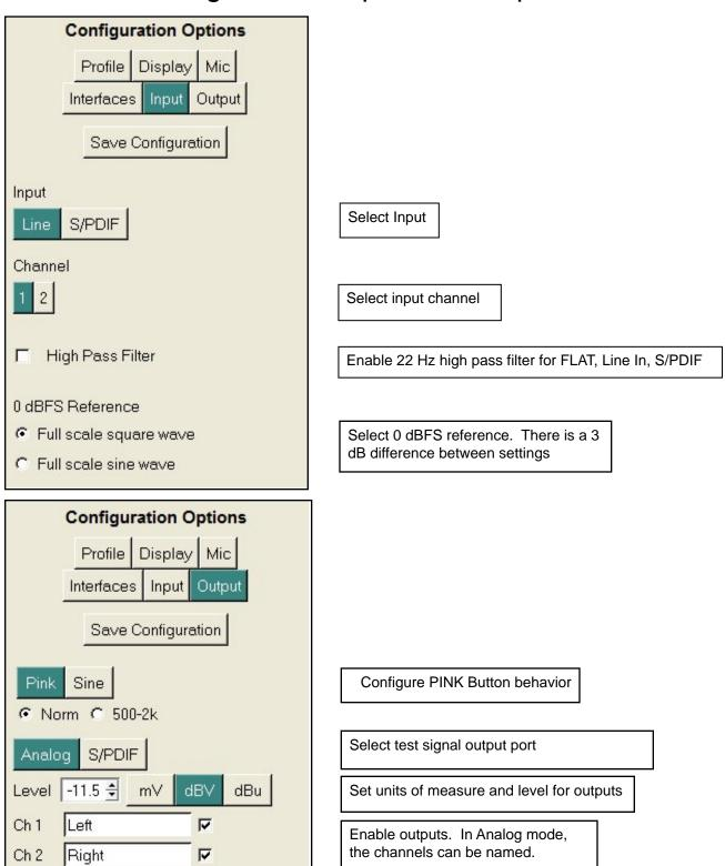
NOTE: The functionality shown on these screens will vary depending on the audio interface. This image shows the configuration for the USBPre. Output voltage is only correct when using an approved interface.
