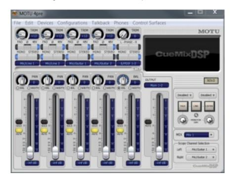
For microphone measurements, load Hardware Preset #1, StudioMicIn
